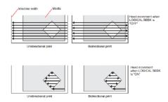
**Note**: If you find that wet ink is affecting the quality (for e.g. in case of higher resolution and high total ink limit), setting Logical Seek to OFF is recommended. This may allow ink to dry between each scan.
