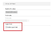
Logical Seek setting controls whether the print head assembly of the printer moves across the full width of the printer or only across the printable data.
